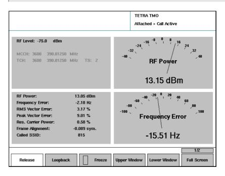
9 To stop the call, push the release button on either the TETRA MS or the 2303 Stabilock.
