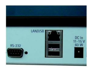
In addition to operating the 2303 Stabilock through its front panel elements, it can also be controlled remotely from a PC through the serial (RS-232) interface or the LAN (local area network).
