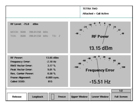
2 If you have set up an individual simplex call, keep the PTT button of the MS pressed.
