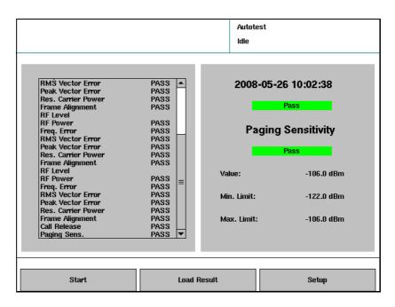
3 In the progress section, highlight a short-form result or test step. Details regarding the short-form result or test step are shown in the details section.
