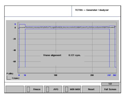
When you are finished with the full-screen burst profile display, return to the Generator / Analyzer menu by pushing the **ESC** button.
