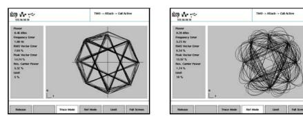
Push Ref Mode and select one of the options from the pull-down menu: Ref Circles for a limit circle around each point of maximum effect, Ref Lines for a cross-hair at each point of maximum effect, Ref Scale for coordinate axes.
