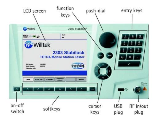
**Menus and softkeys** The most important elements are the menus displayed on the LCD screen, and the six softkeys below the screen. The screen always displays a menu with either input fields or results or both, and a description of the current functions of each of the six softkeys.
